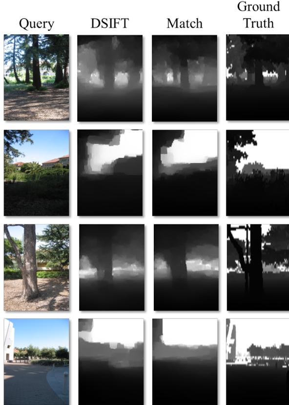
Figure 8: **Qualitative example results on the Make3D benchmark [30].** Single image depth estimation results using the Depth Transfer approach of [14]. Left to right: The input image; depth estimated using the standard DSIFT representation; depth estimated using our match-aware scale propagation; the ground truth. See text for more details.
