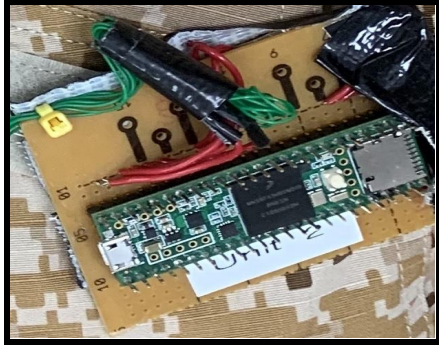
Figure A5. A microcontroller, Teensy 3.6, used for fsr, piezo signal collection.
