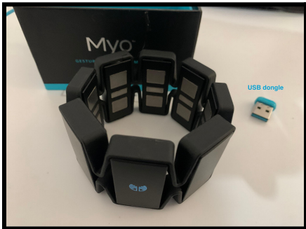
Figure A3. A Microcontroller, Myo-armband. used for emg signal collection.
