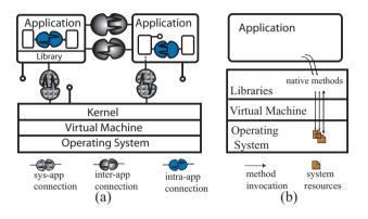
Figure 2. (a) The  $\mu$ KVM runtime overview and (b) J2SDK Runtime
