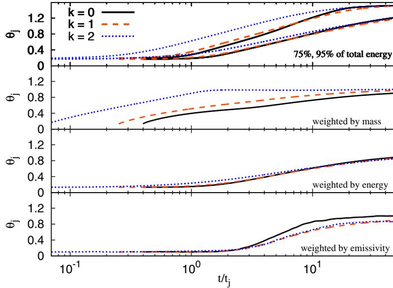
**Figure 6.** Evolution of the jet half-opening angle  $\theta_j$  as a function of time for different  $k$  values. The various panels give  $\theta_j$  derived based on the angle-integrated mass, energy (excluding rest mass), and emissivity (at  $10^{17}$  Hz). Also plotted is the evolution of  $\theta_j$  computed as the characteristic angular scale containing 75% or 95% of the total energy (excluding rest mass).
